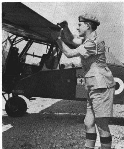
Cpl. Smith, an aircraft crewman adjusts a trim tab on an Auster before Exercise "Trojan Horse"
