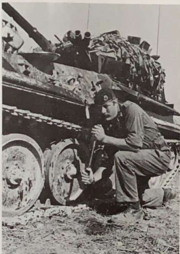
Tightening the tracks (Scorpion) Cpl. Terence Skelly working up a thirst during the autumn exercise in the Mosel Valley
